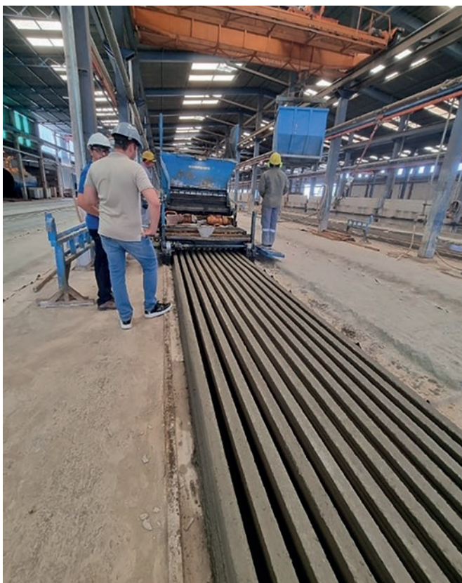
Casting of 210mm thick I-beams with Nordimpianti's Slipformer machine
