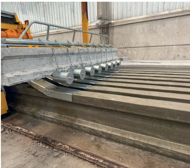
I-beams produced by Nordimpianti's Slipformer machine
