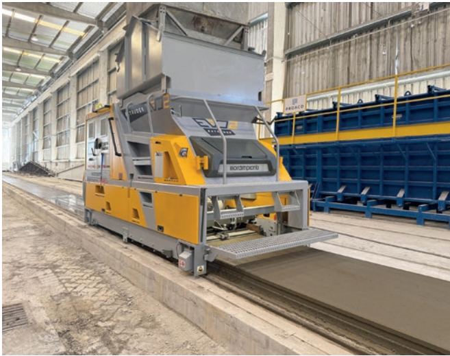
Top surface finish with Nordimpianti's EVO2 extruder casting machine
