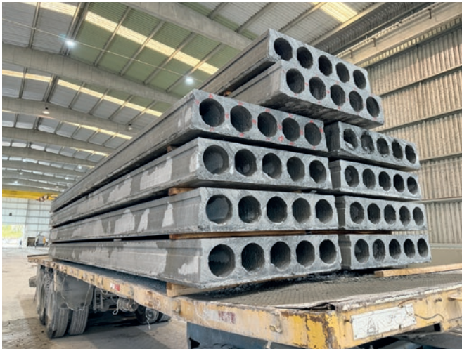
5 hole hollow core slabs cast by Nordimpianti's EVO2 extruder
